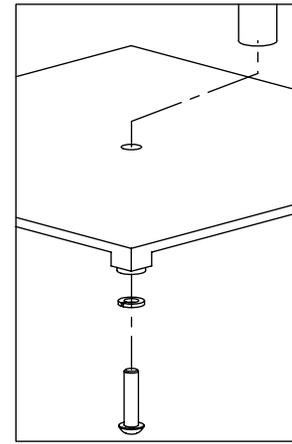
1 SECURE UPRIGHT TO BASE WITH SCREW AND WASHER AS SHOWN.
