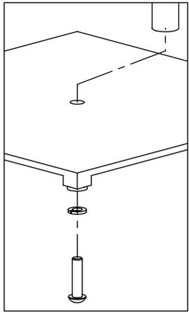
1 SECURE UPRIGHT TO BASE WITH SCREW AND WASHER AS SHOWN.
