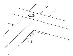
2 SCREW IN WING-NUT AFTER UNFOLDING
