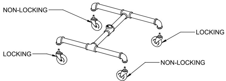
SCREW IN THE CASTERS TO THE BASE AS SHOWN USING PROVIDED WRENCH.
